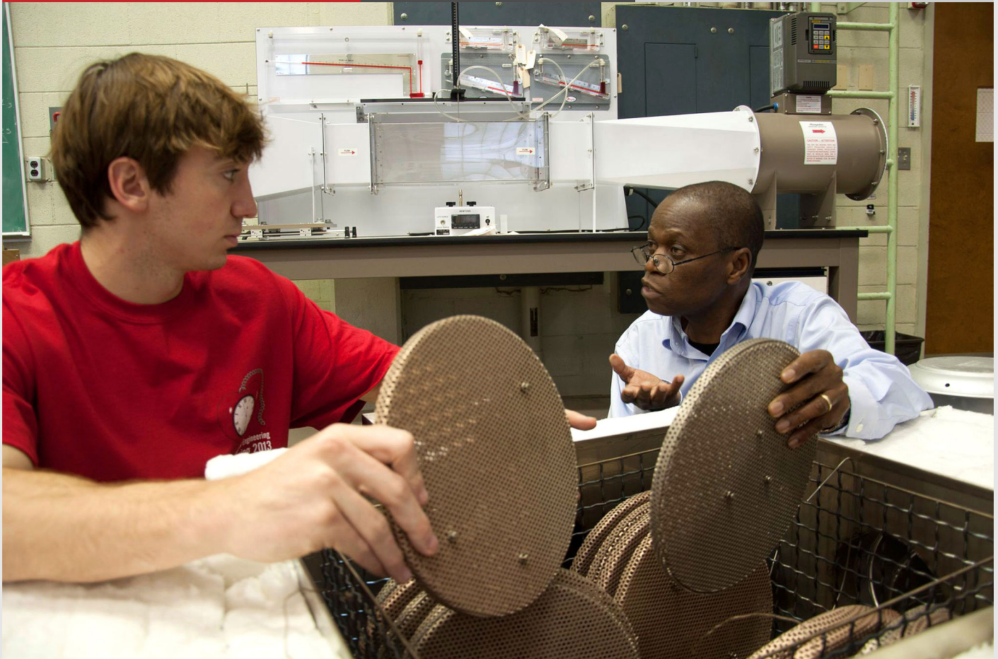
William Kisaalita, right, a biological and mechanical engineering professor in UGA's College of Engineering, works with Ryan Brush, an undergraduate student worker in his lab, on the milk cooler used in his refrigeration project in Uganda.
